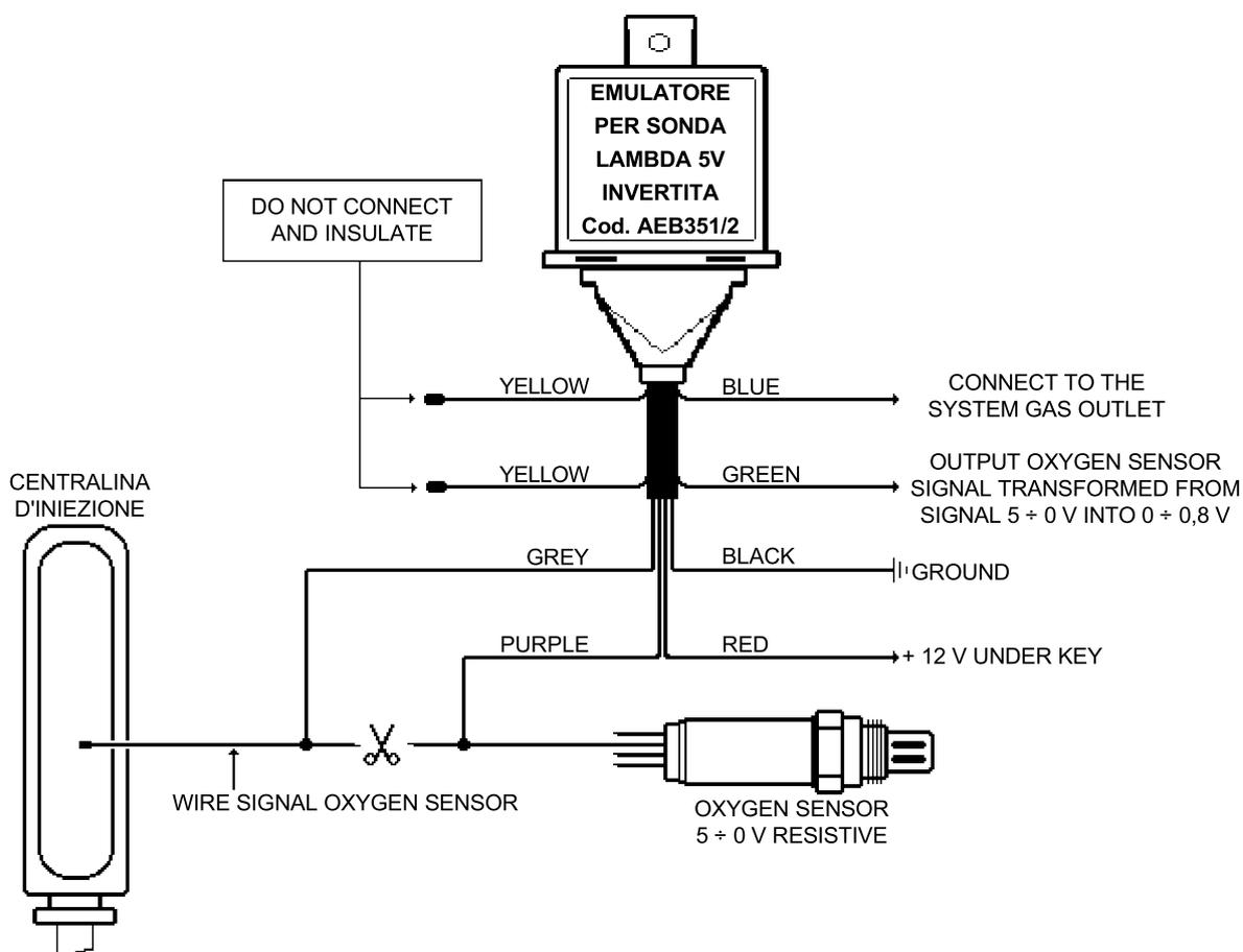
The AEB351/2 emulator switches on during the gas running and switches off during the gasoline running, thus automatically resetting the connections to the car original electrical system; this applies also in case of failure, thus allowing the user to drive the car with gasoline and reach a service point for checking.
