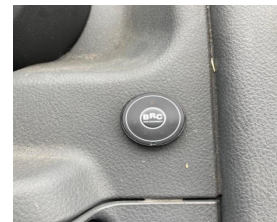
Reinstall the switch in its location.
