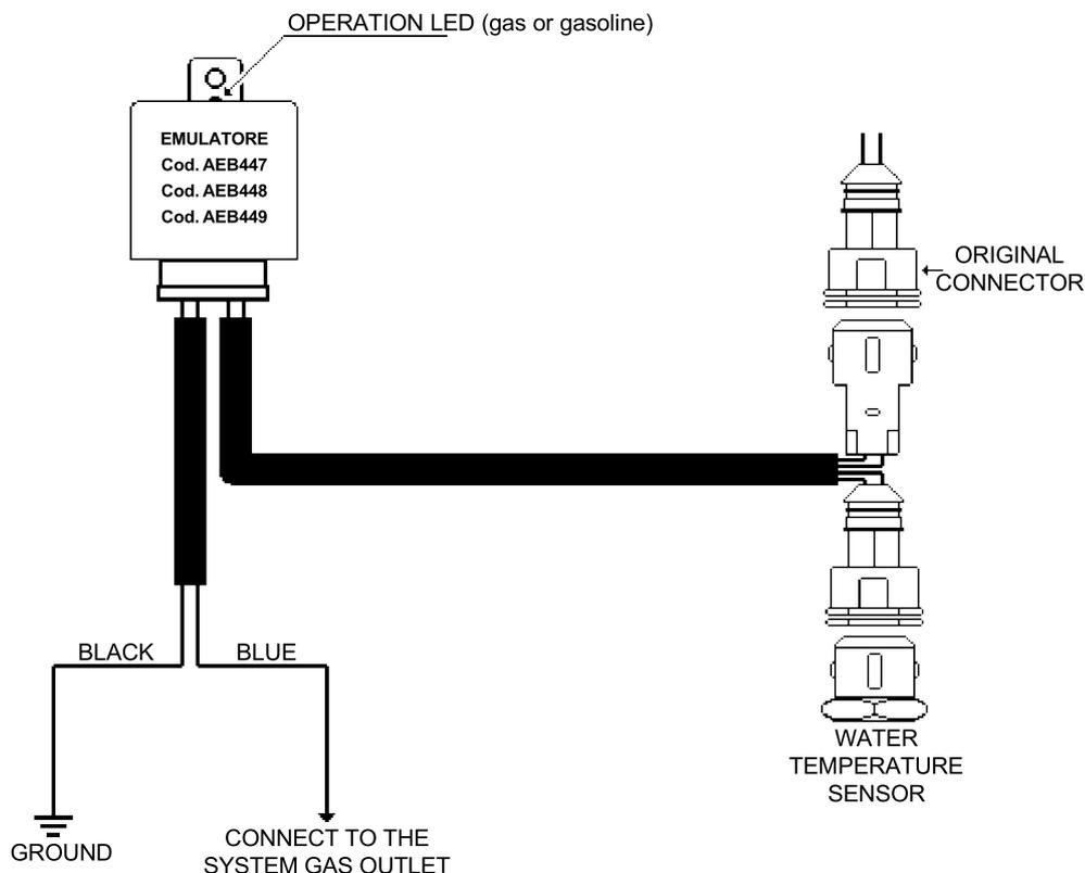
The AEB447, AEB448 and AEB449 emulators switch on during the gas running and switch off during the gasoline running, thus automatically resetting the connections to the car original electrical system; this applies also in case of failure, thus allowing the user to drive the car with gasoline and reach a service point for checking.
