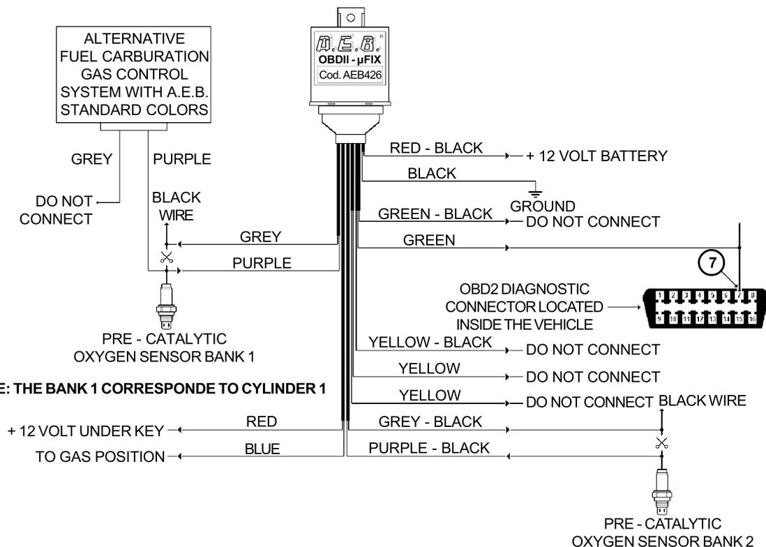
AEB426 switches on during the gas running and switches off during the gasoline running, thus automatically resetting the connections to the car original electrical system; this applies also in case of failure, thus allowing the user to drive the car with gasoline and reach a service point for checking.
