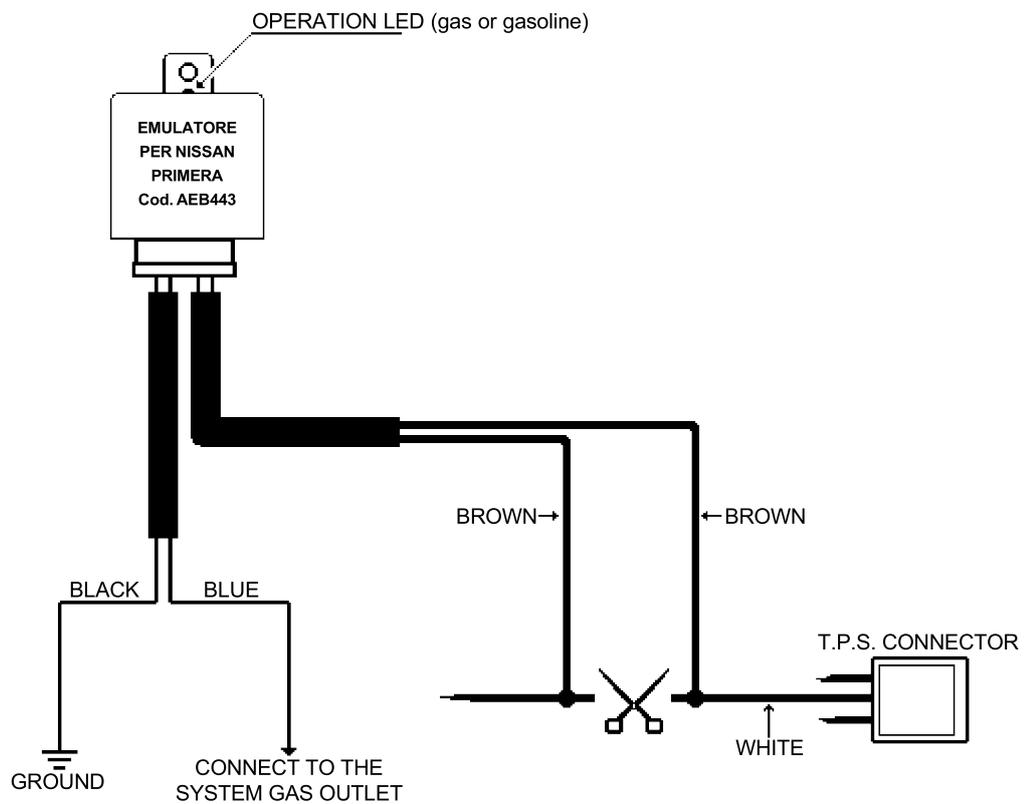
The AEB443 emulator switches on during the gas running and switches off during the gasoline running, thus automatically resetting the connections to the car original electrical system; this applies also in case of failure, thus allowing the user to drive the car with gasoline and reach a service point for checking.
